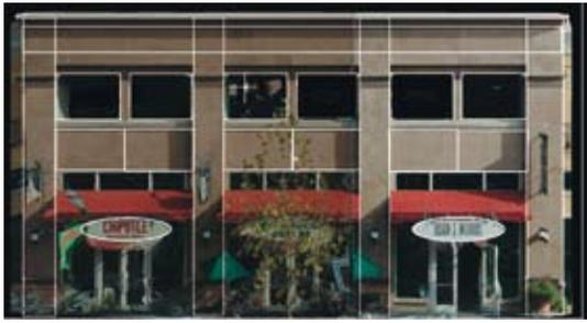
One common usage of point cloud data in CloudWorx is to trace over the point clouds to create dimensionally correct 2D or 3D wire frames for building elevations, model extrusions, etc. Several CloudWorx commands make this easy.
